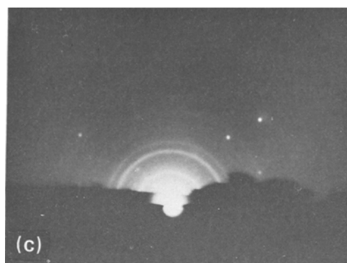
Figure 2 Reflection electron diffraction patterns taken at 80 kV of anodic films formed at 6 volts on V, Nb, and Ta. That on V (a) is crystalline, corresponding to a still unidentified lower oxide. That on Nb (b) is amorphous and therefore of unestablishable stoichiometry. That on Ta (c) is tentatively identified as a mixture of TaO_z and \delta -Ta-O.
